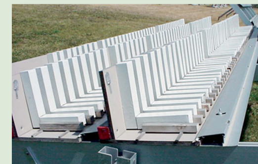
"L-Joint" visual appearance environmental test
